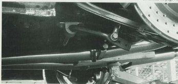
The thicker rear anti-roll bar also boasts three different levels of adjustability for more precise roll control.
