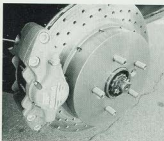
Because the Z-car's emergency brake is integral in the hat of the rear disk, they are often not upgraded beyond brake lines and pads. KVR was able to machine an iron lining for the aluminum brake hat. The result is a 12.5-mch disk where the stock 11.6-mch disk used to be.
