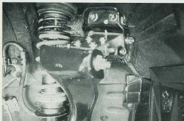
The Stilen adjustable front A-arm assembly allows for camber changes on the Z-car. This allows better alignment when larger wheels and tires are put on the car, as well as more precise handling.
