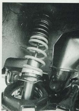
The Ground Control springs in the rear offer the same advantages as the front springs, with the stock strut still in place for the on-board adjustability, and the Eibach main and tender spring.
