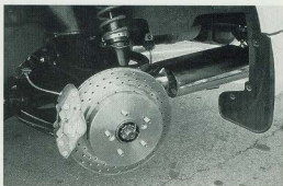
The rear brakes are also from KVR, with SMC stainless steel lines. The Ground Control strut is visible behind the new rear disk.
